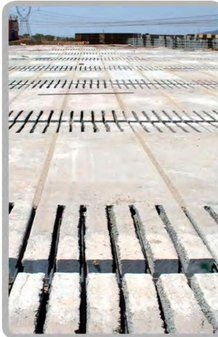
The Topfloor slab can be made composite with the supporting beams to increase the overall structural depth of the supporting beams.
